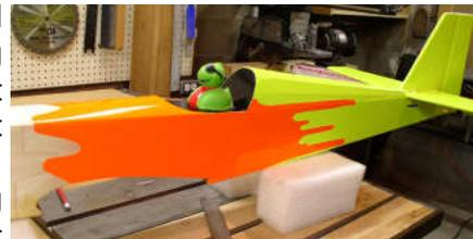
After the first section is covered and trimmed it is time to start adding the additional colors of the design. I like to first rough fit the covering over the area, and hold it in place with tape. A water base (non-permanent) marker can be used to draw the design free hand. Then the design can be cut out, wipe off the marker
