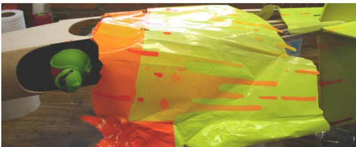
It is not often that a plane outlives it's colors, but I should have not underestimated the fluorescent colors ability to fade -just as promised on the package. In fact the first clue should have been the fading on the first turn of the new roll- right from the store shelf. Overtime some of the colors actually faded away to nothing. Although never crashed, it started to look so bad the plane was back shelved.
