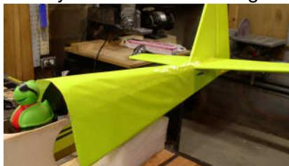
Starting from the rear of the plane, the tail feathers and rear section are first to get covered. A regular hair dryer will get the covering nice and soft to get a good fit without kicking the glue. After pulling, fitting and tacking it down, a covering iron and high heat gun will kick the glue and shrink the coating. The better the fit before shrinking the better the final fit will be.
