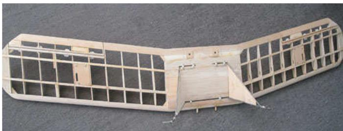
As you can see the gear came out fine I did the soldering while the wires were mounted to the bottom wing. Made for a fine jig. The wing doesn't have much dihedral it's the swept back that makes it look like dihedral in the photo
