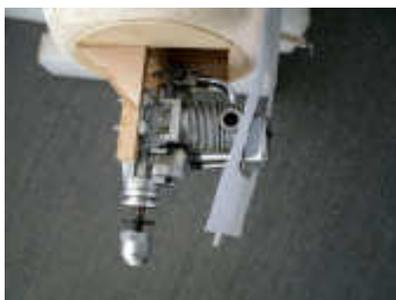
I usually just eyeball where the holes goes for the glow igniter and the high and low speed carb needles go on the cowl but I have, in the past, used the same method I use for the engine cylinder head to locate those..
