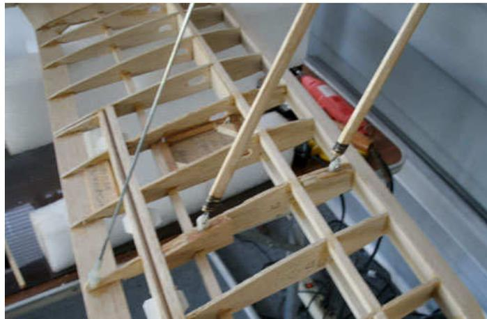
After I had those bending, soldering and hole making jobs done I mounted the wings on the fuse and made the four wing struts and the two aileron push rod connectors, Theoretically, if you make the two front struts and the two back struts the same you shouldn't have to keep track of which goes where and the the wings will be equal distance apart and the incidence according to the plans. The same thinking goes for the aileron connectors too, but there is adjustment on the connectors.
