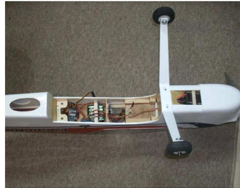
The photo on the left shows the plane viewing through the wing saddle. The motor controller is in the space given over to
