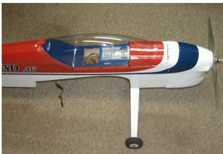
4000 mah six cell Li-po battery. What you can't see is two slots I cut in the canopy at the back for extra cooling for the battery.
