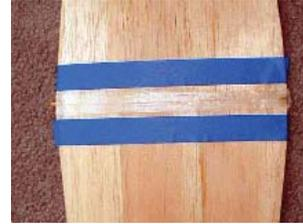
One word of warning, though. If you use alcohol to thin your epoxy, as I do, it will probably leak under the tape. The good part is that it also soaks into the wood better, so it's less likely to show.
