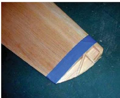
And while it isn't quite paint masking, you can use masking tape to control the spread of excess epoxy when applying wing center-section tape.
